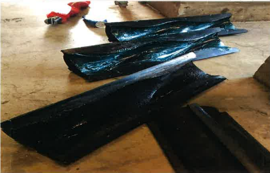
Grass Valley WWTP Primary sludge pumps re-build. The photo shows worn out “stators” due to the high volume of grit pumped by the primary sludge pumps during the 2019 storm events, along with the new stators (greased). The stator is shown on the diagram as Item # 601. Both the rotor and stators were replaced on both Primary sludge pumps post-2019 storm surge by the Mechanical Maintenance Department.
