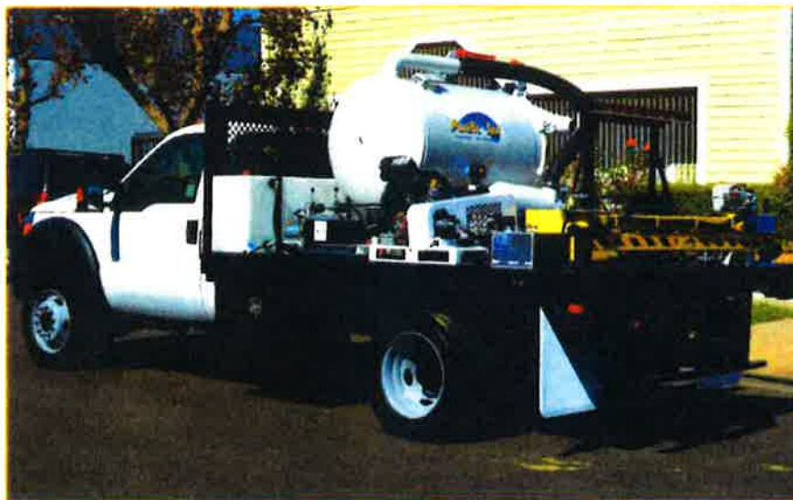
PV-253 Valve & Vac Unit Mounted on an F-450 Flatbed Truck
